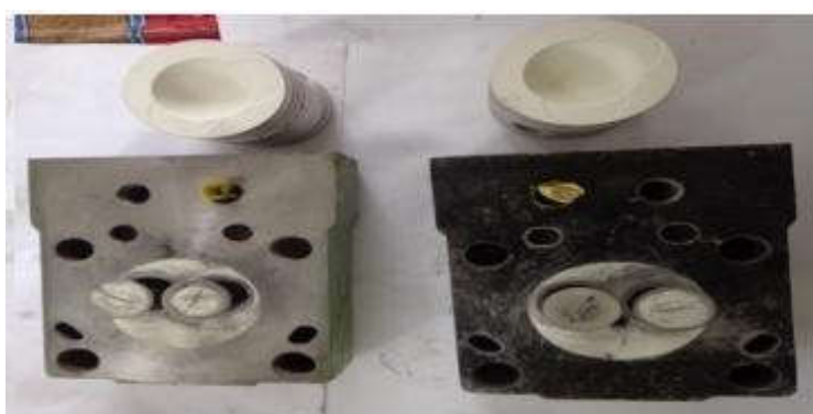
Figure.3. Engine Piston, Head & Valve without Coating of YSZ
