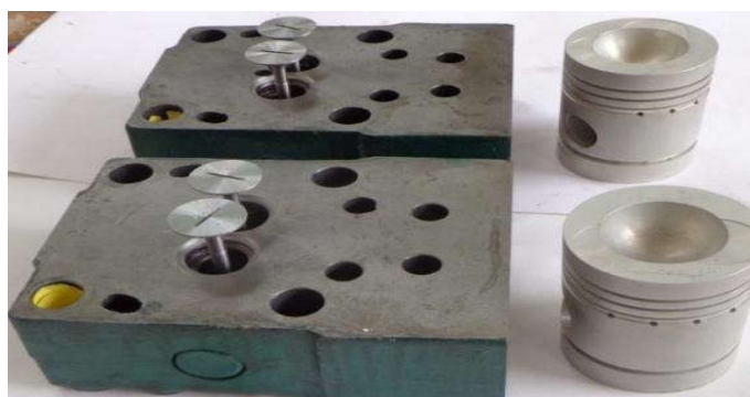
Figure:2 Engine Piston, Head & Valve without Coating
