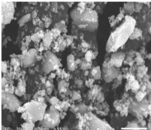
The morphology and particle size of the catalyst play very important role in its photocatalytic activity. SEM image of 0.75 wt.% of N- TiO<sub>2</sub> is shown in Fig.2. The image showed irregular tiny clusters composed of large numbers of nanoparticles with lower aggregation and better distribution. From the SEM micrographs it can be inferred that aggregation is decreased greatly due to doping.
