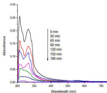
The spectrum representing the degradation of Malathion using this sample was represented in Fig. 3. The absorbance gradually decreased as time passed and became almost zero after 180 min indicating complete degradation of Malathion under direct sunlight in summer season.
