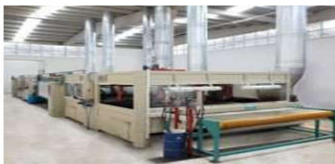
Fig: 1 Auto Spray machine in Tannery
