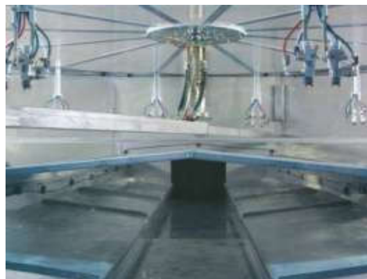
Fig.3: Carouse 1 plate with Spray gun
