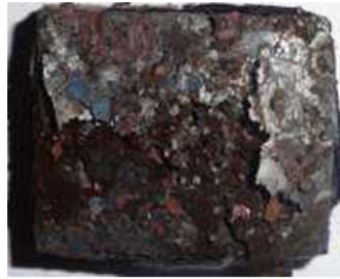
Figure 1: Macrographs of uncoated bare boiler T22 steel subjected to cyclic oxidation in air for 50 cycles at 700°C
