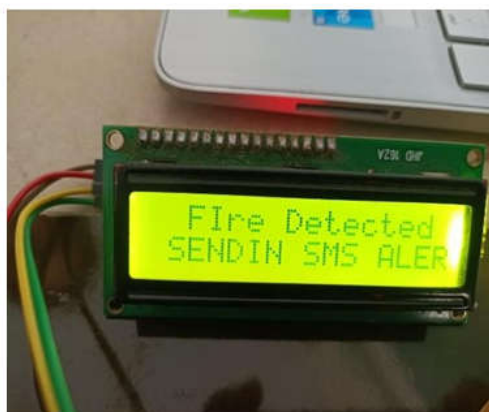
Fig. 2 Flame sensor output along with GSM Module
