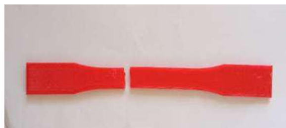
Figure No.1: Fracture of PLA Specimen after Tensile test
