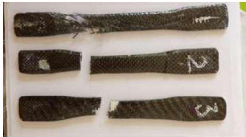
Figure No.2: PLA wrapped with carbon fiber fabric after the tensile test
