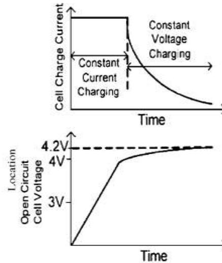
Figure 3. Typical Lithium Ion charging characteristics [4]
