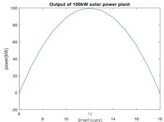
Figure 1. Matlab simulation for 100kW solar power plant.
