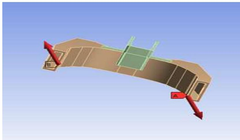
**Fig 3. Cornering Forces Acting On the Swingarm.**
