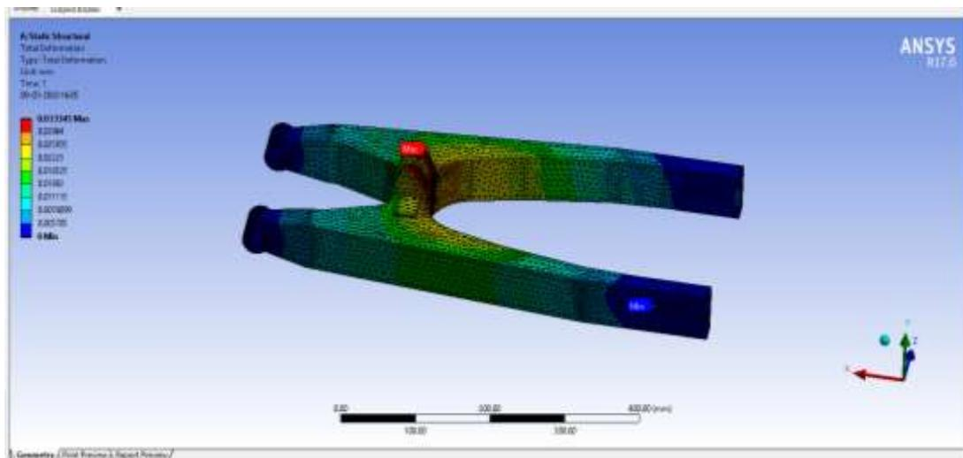
Fig 9. Deformation Of The Swingarm With AISI 1020 As Material
