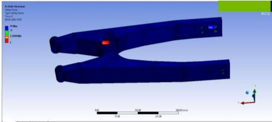
Fig 12. Factor of Safety of The Swingarm With AL7075 As Material
