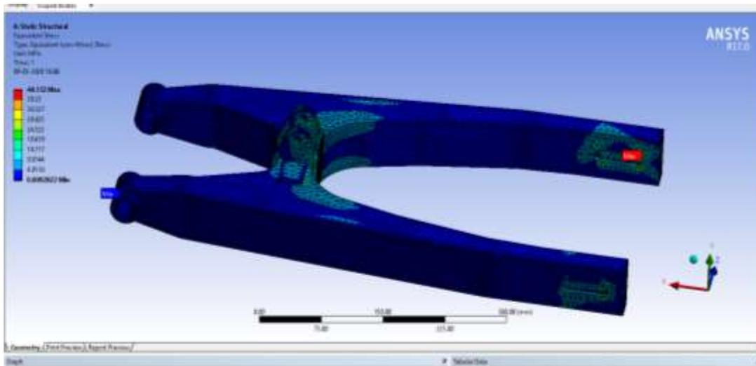
Fig 8. Stresses Developed In Swingarm With AISI 1020 As Material
