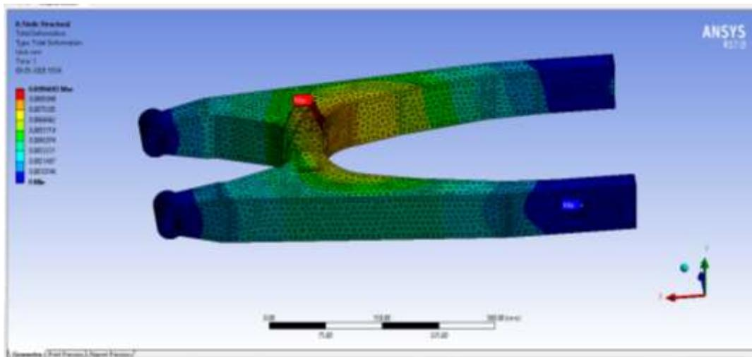
Fig 14. Deformation of Swingarm With AL7075 As Material
