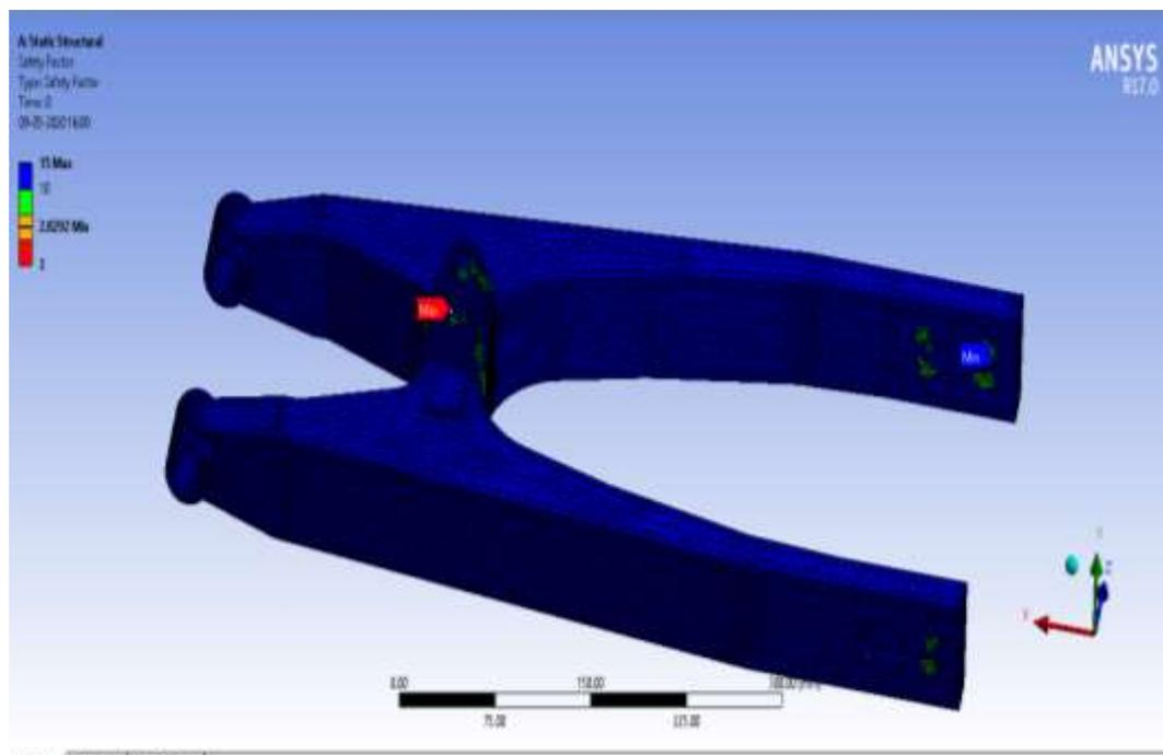
Fig 7. Factor Of Safety of the Swingarm With AISI 1020 As Material
