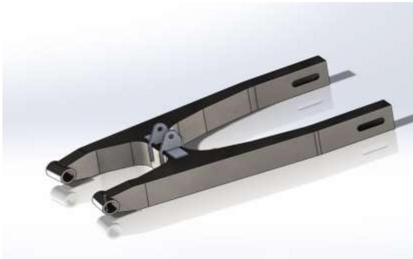
**Fig. 1 Model of the Swingarm.**
