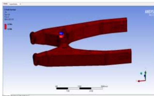
Fig 11. Life of the Swingarm with AL7075as material
