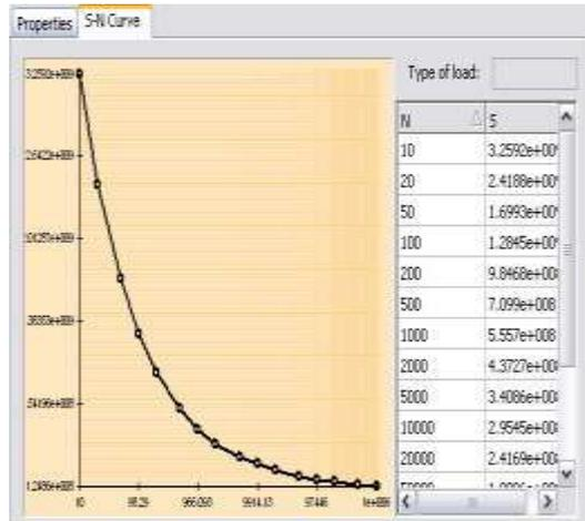
Fig 5. S-N curve of AISI 1020
