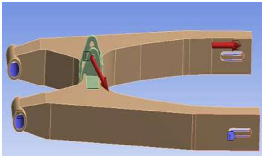
**Fig 2. Forces That Were Acting On the Swingarm**
