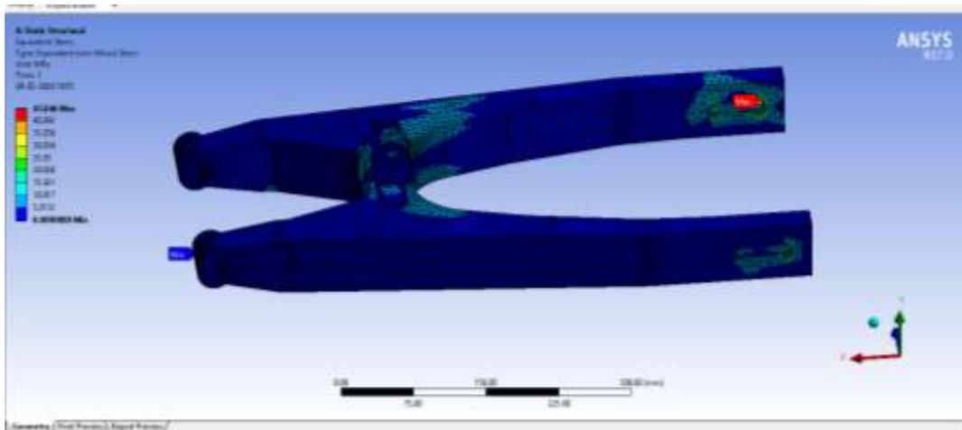
Fig 13. Stresses Developed In Swingarm With AL7075 As Material
