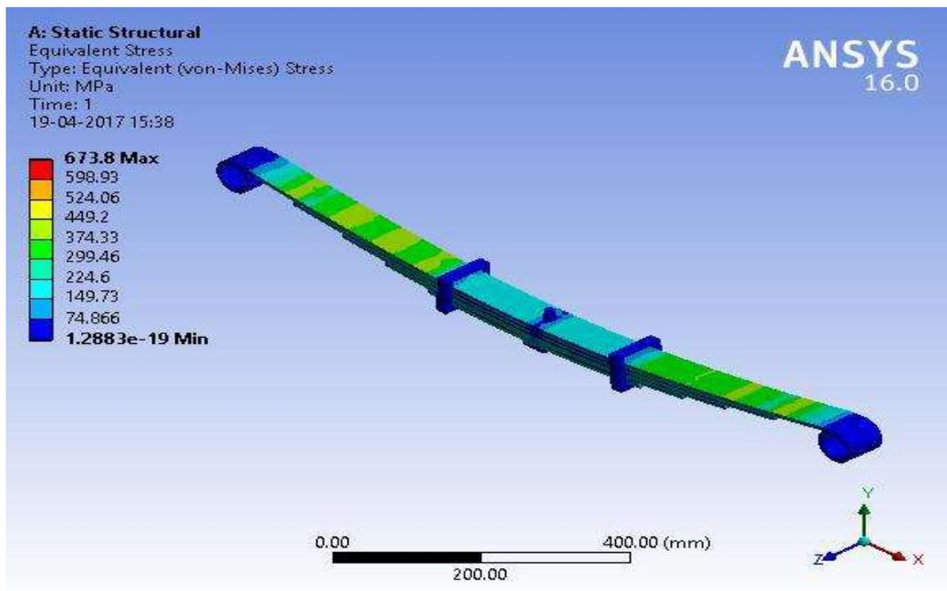
**Fig 3. Equivalent stress of Carbon Fibre**
