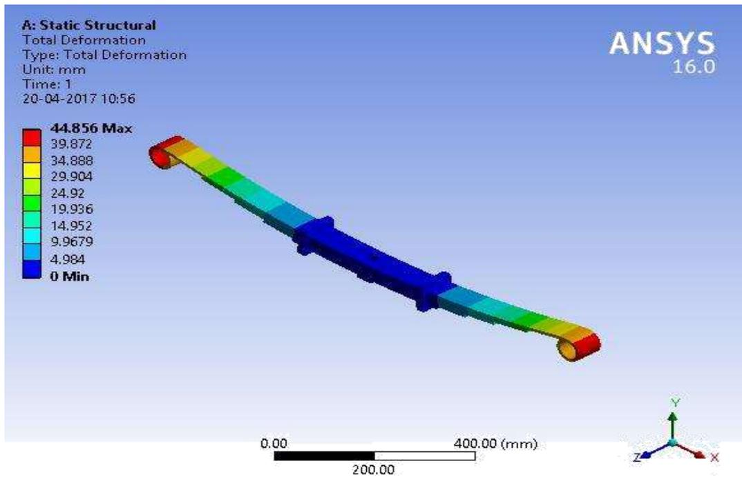
**Fig 12. Total Deformation of Aluminium oxide**
