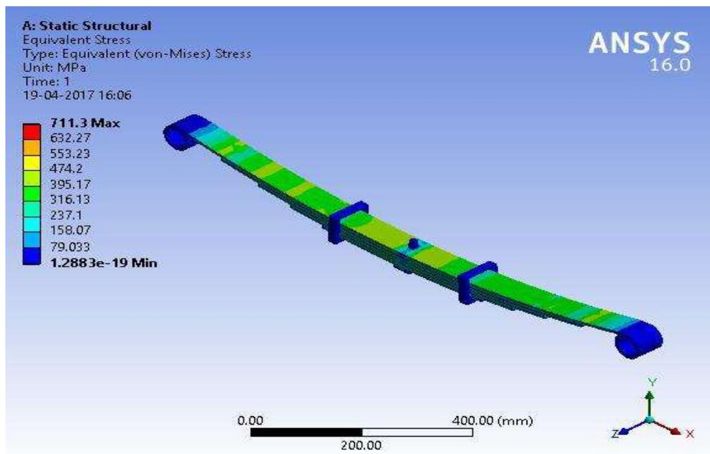
**Fig 5. Equivalent stress of Co-Cr-Ni Alloy**
