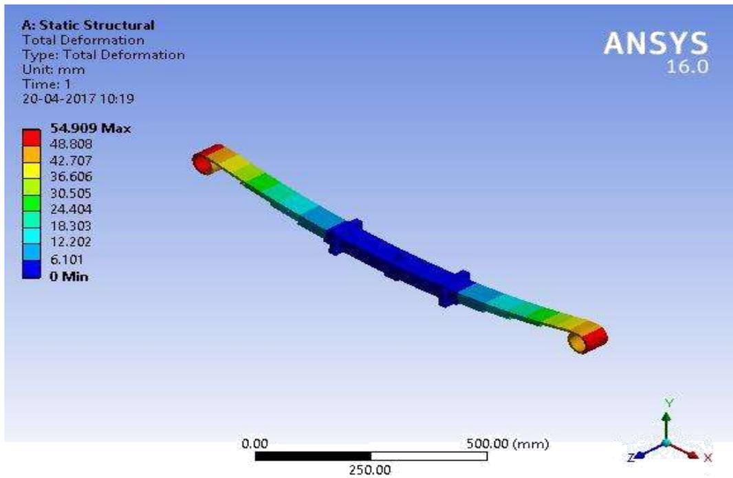
**Fig 6. Total deformation of Co-Cr-Ni alloy**
