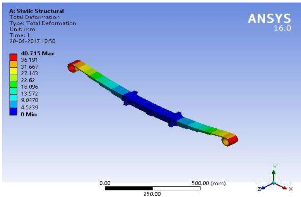
**Fig 8.Total Deformation of Silicon Carbide**
