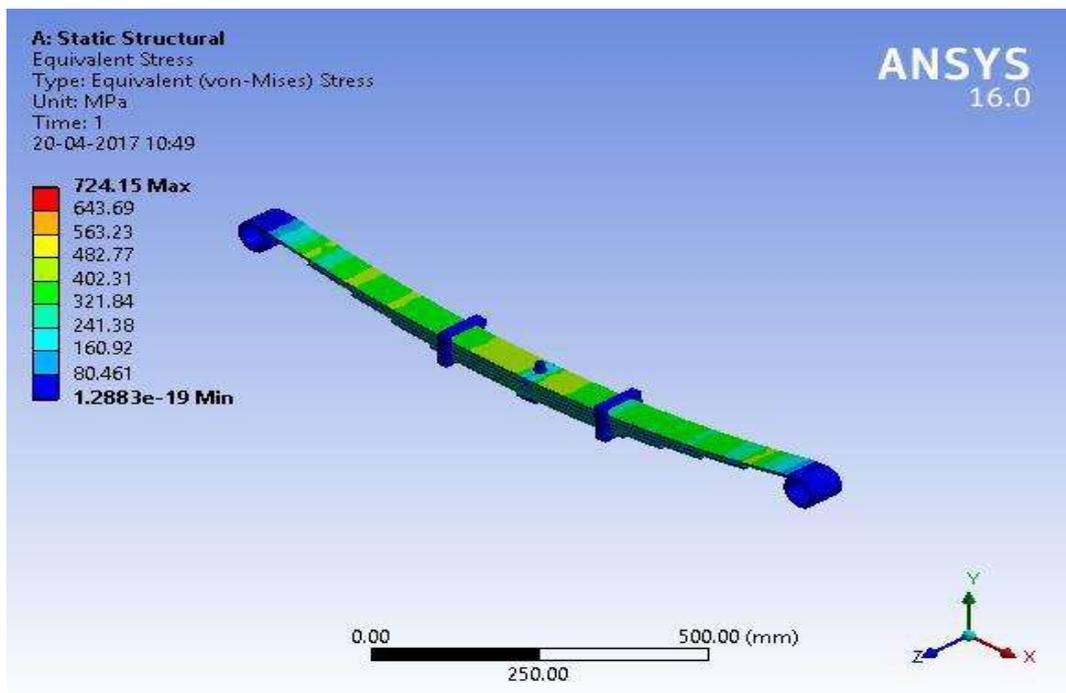
**Fig 7. Equivalent stress of silicon carbide**
