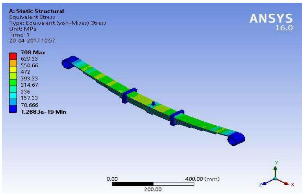
**Fig 11. Equivalent stress of Aluminium oxide**
