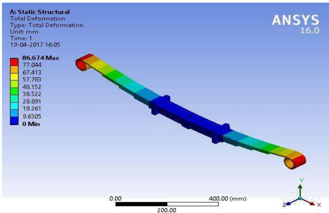
**Fig 4. Total Deformation of Carbon Fibre**
