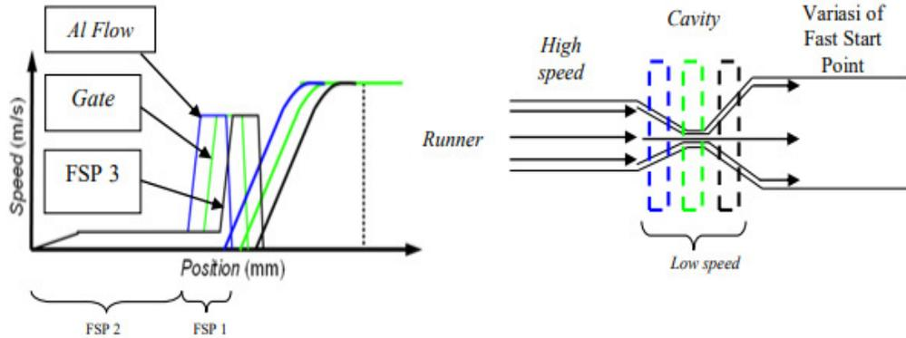
**Figure: Fast start point on the gate of HPDC process on compressor product.**
