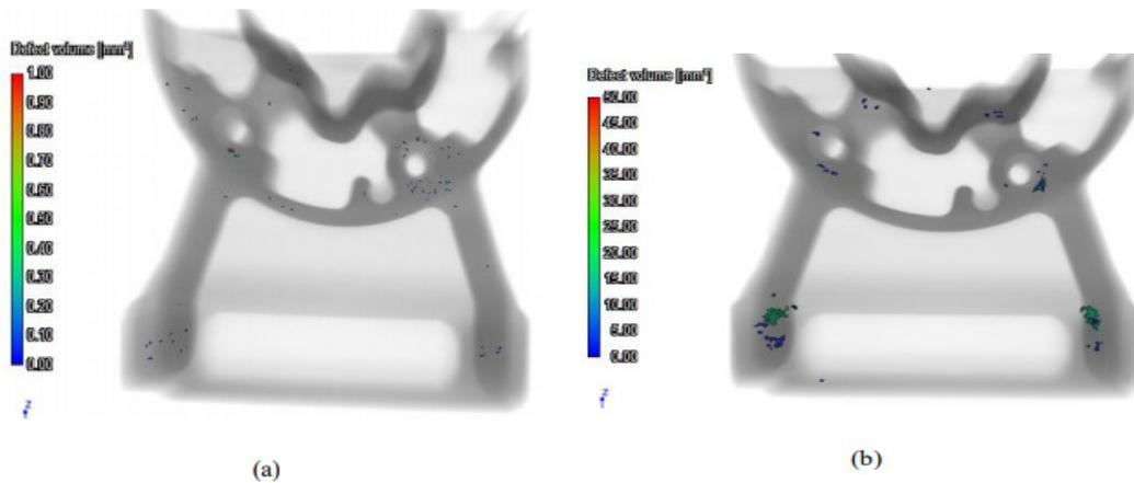
**Figure: Radiographic observation image: (a) minor defect, (b) major defect.**
