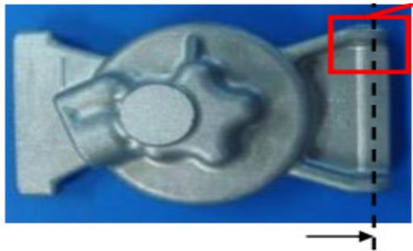
**Figure: Sample position to examine the microstructure.**
