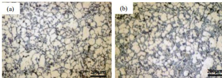
**Figure: Microstructure of block compressor with HPDC parameters of: (a) 3.97 m/s with 293 mm, (b) 4.97 m/s with 313 mm**
