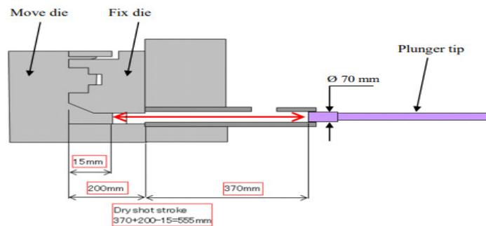
Figure: Injection system of molten Al alloy into metal mold using HPDC process
