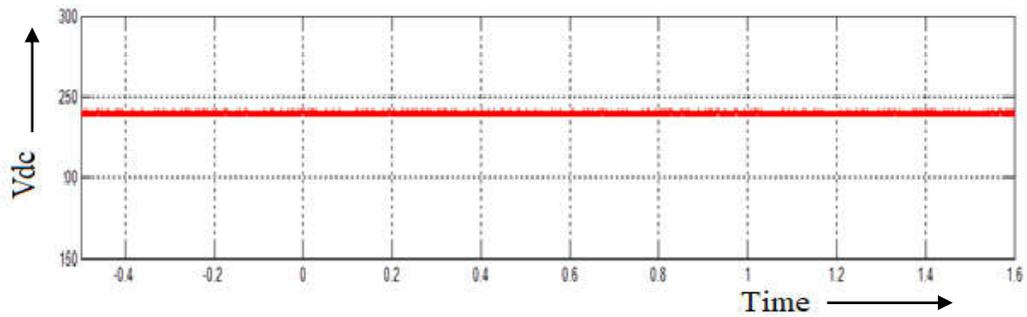
Fig.10 Voltage available at DC link
