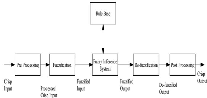
Fig.44. Block diagram of fuzzy control system
