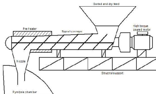
**Fig.2 Continuous Feed Mechanism**
