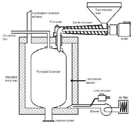
Fig.3 Pyrolysis Chamber Assembly
