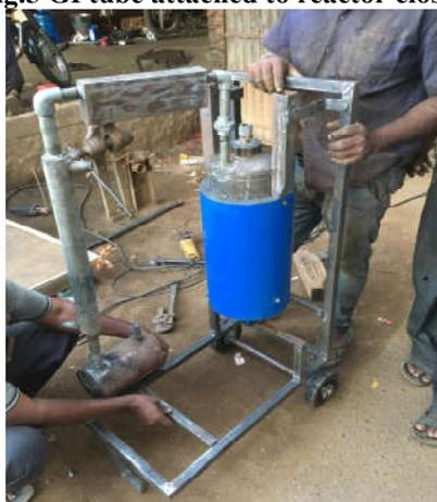
**Fig.6 GI tube attached to the condenser.**
