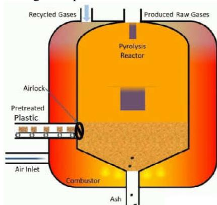
**Fig.1 Pyrolysis Process**
