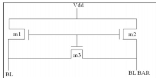
**Fig.6. Pre-charge circuit**
