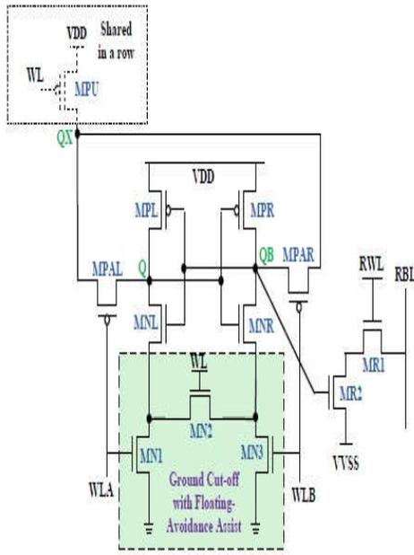
Fig 2 Proposed 11T-2 cell Schematics
