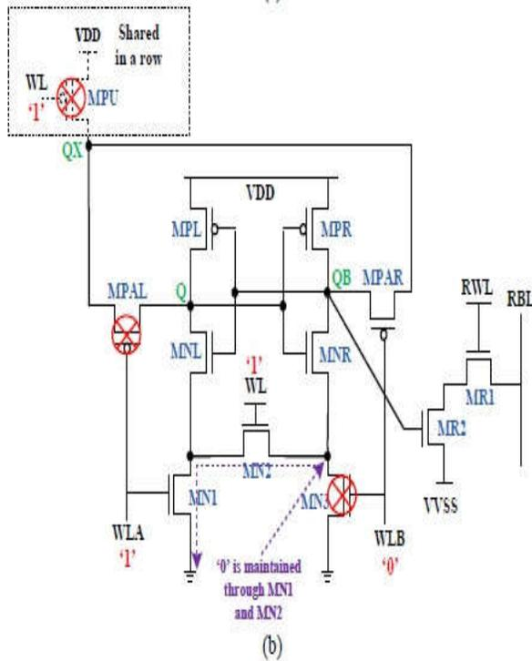
Fig 4 Column Half-select cell under write '0' operation in (a) 11T-1 (b) 11T-2 cell
