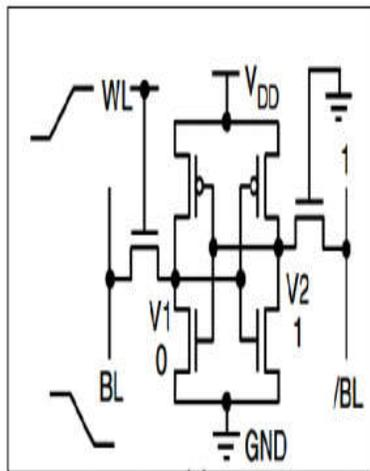
**Fig.5. Design of Single Bit-Line SRAM using Adiabatic Logic**
