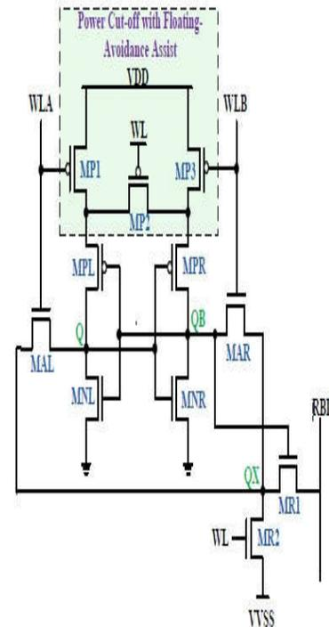
Fig 1 Proposed 11T-1 cell Schematic
