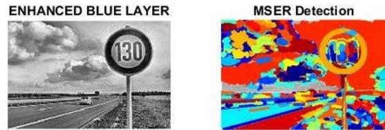
Figure 4.11 MSER Features extracted for Blue Layer
