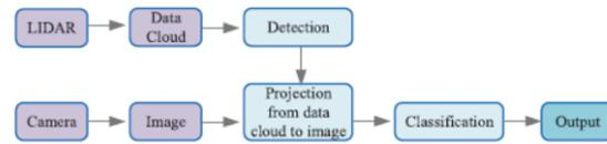
(e) LIDAR and Camera based structure
