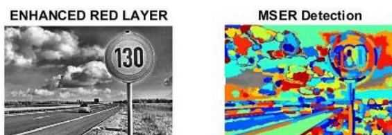
Figure 4.9 MSER Features extracted for Red Layer
