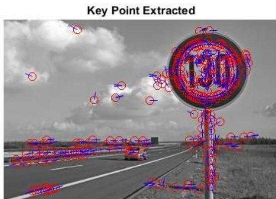
Figure 4.8: Key Point Extracted image using SIFT
