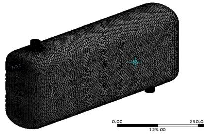
Fig 4: meshing of modal of feed water heater
