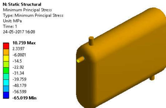
Fig 7 :Max minimum Principal stress is 10.756 mpa in feed water heater
