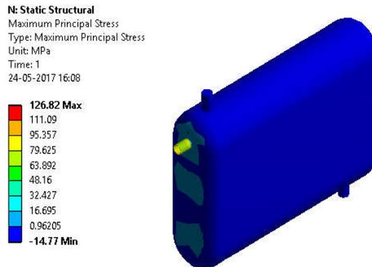
Fig 6 :max maximum principal stress is 126.82 mpa in feed water heater
