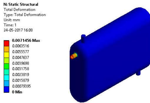
Fig 8 : max total deformation is 0.0071456 in feed water heater
