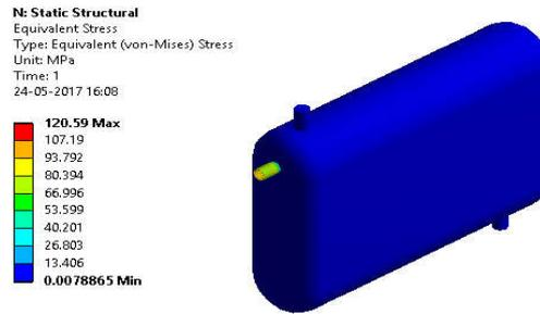
Fig 5 :max equivalent stress is 120.5 mpa in feed water heater
