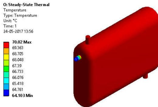
Fig 9: max temperature is 70.02 °Cin feed water heater
