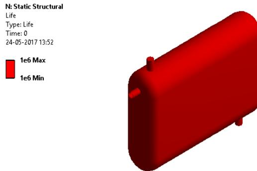
Fig 11: life estimation is 100000 cycles is feed water heater
