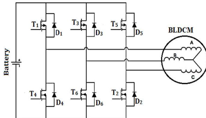
Fig.4: Inverter Circuitry for BLDCM
