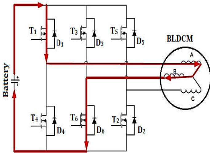
Fig. 5. Current Flow during Motoring
