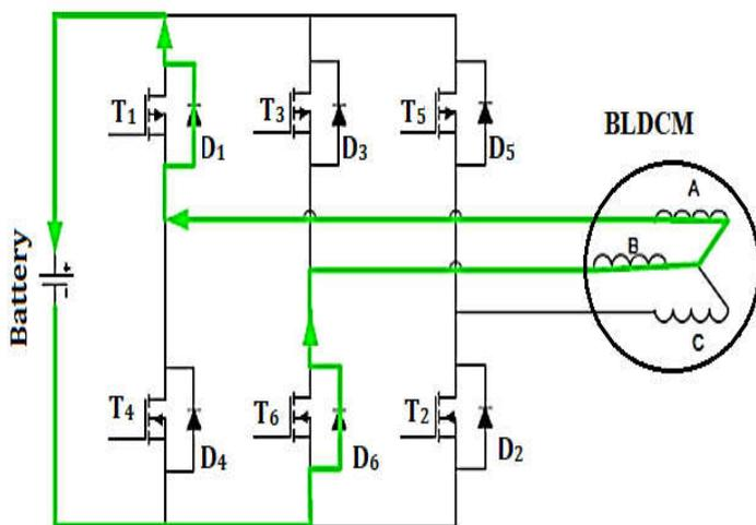
Fig. 6. Current flow during Regenerative Braking
