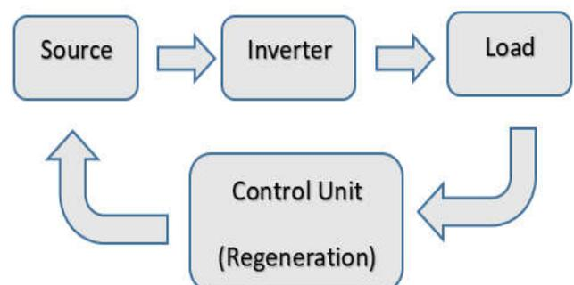
Fig.1. Block Diagram for Typical Regenerating Scheme
