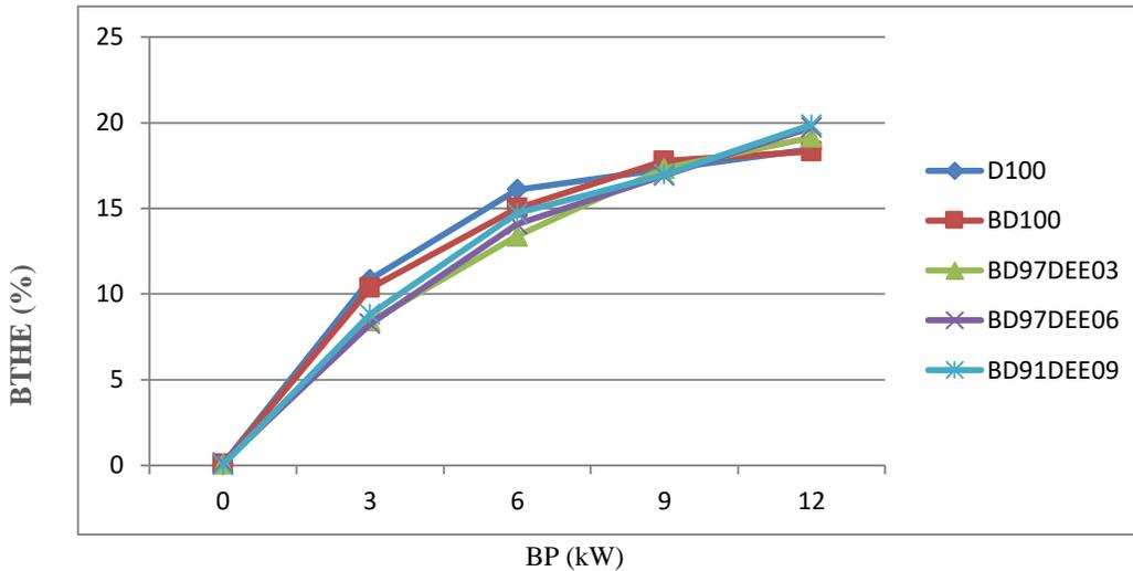
Figure 11: Variation of brake thermal efficiency (%) with brake power (Kw)
