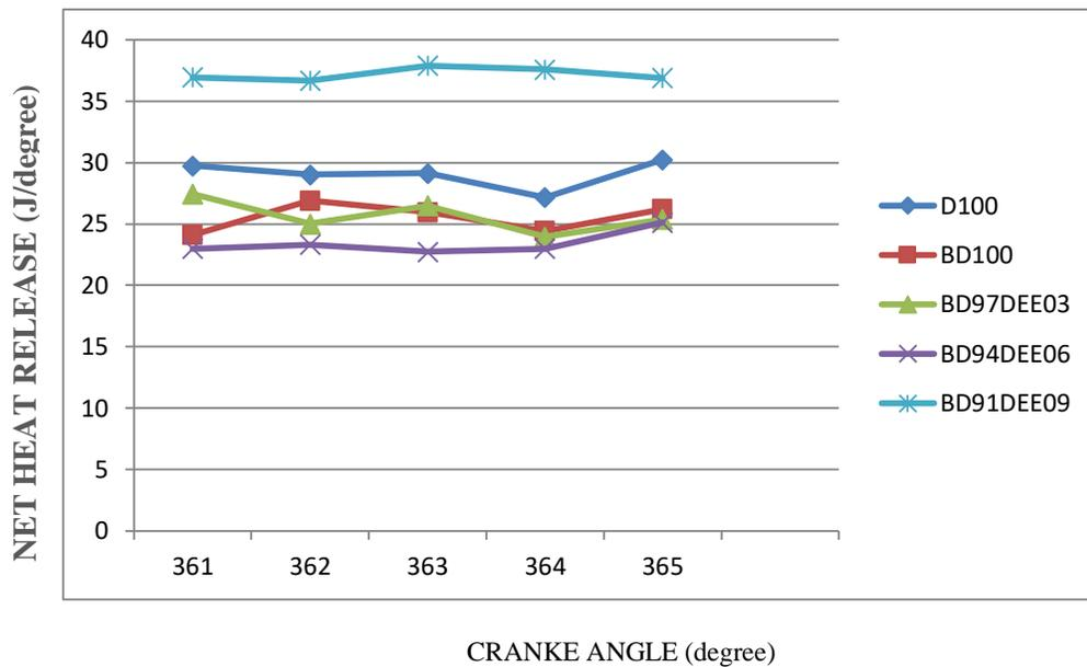
Figure 6: Variation of net heat release rate by crank angle
