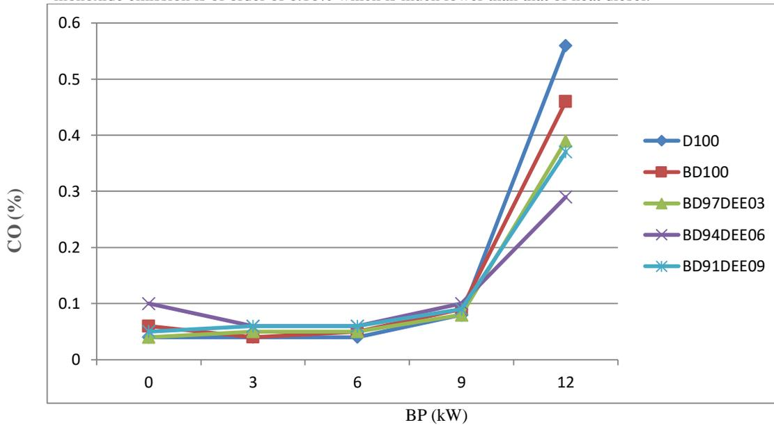
Figure 8: Variation of carbon monoxide emission with brake power
