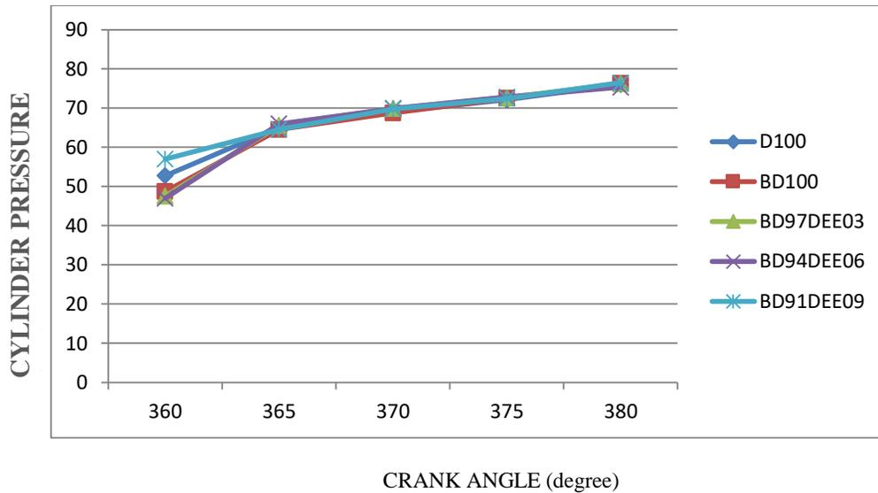
Figure 5 Variation of cylinder pressure with crank angle
