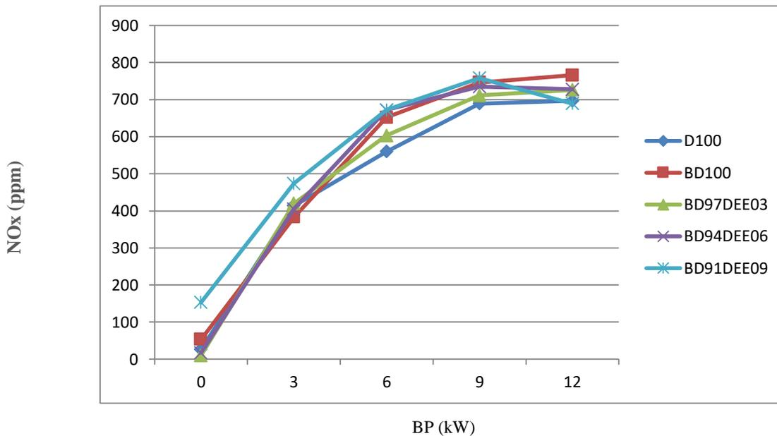
Figure 10: Variation of oxide of nitrogen emission with brake power
