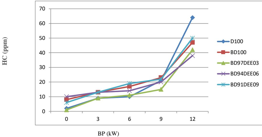
Figure 9: Variation of unburnt hydrocarbon emission with brake power
