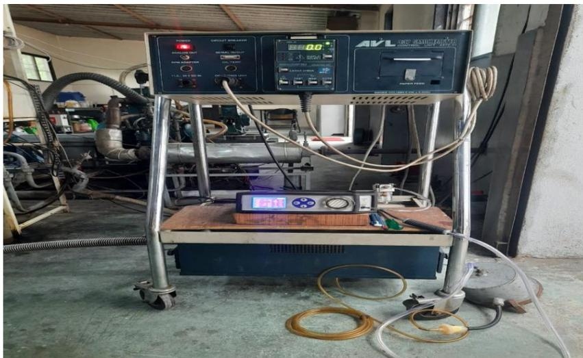
Figure 4: AVL Exhaust gas analyzer
