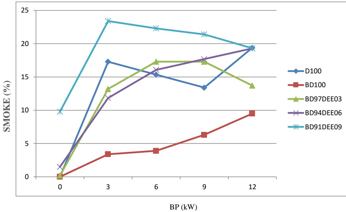
Figure 7: Variation of smoke opacity with brake power
