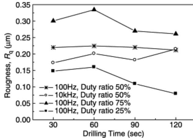
Fig. 2. Surface roughness,  $R_q$ , as a function of micro drilling time. [2]
