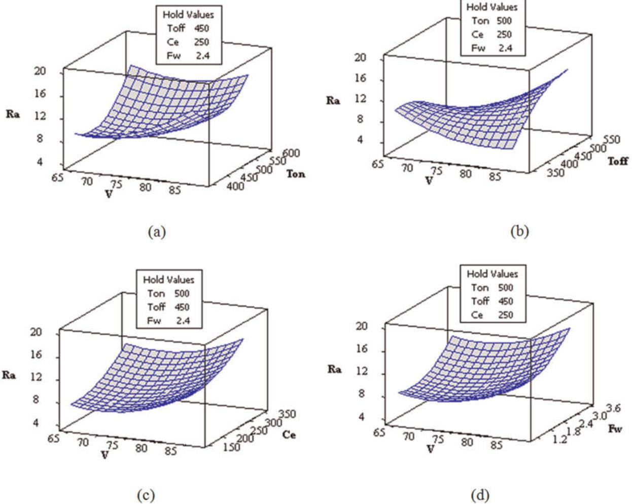
Figure 3. Response surface plot of Ra with (a) applied voltage (V) and pulse on-time (Ton), (b) applied voltage (V) and pulse off-time (Toff), (c) applied voltage (V), electrolyte concentration (Ce), (d) applied voltage (V), and wire feed velocity (Fw).[3]
