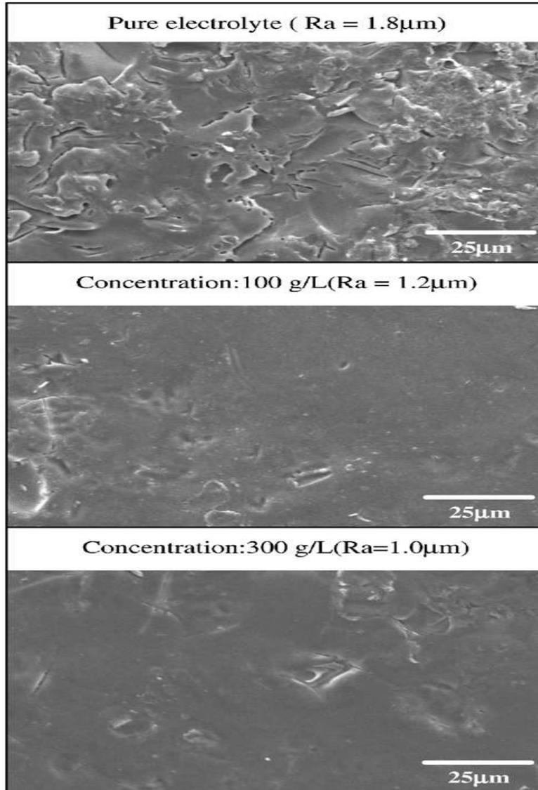
Fig. 1 SEM micrographs of surface at different abrasive concentrations. [1]
